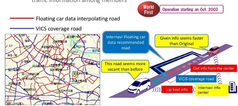
VICS: Vehicle Information and Communication System (National infrastructure)
