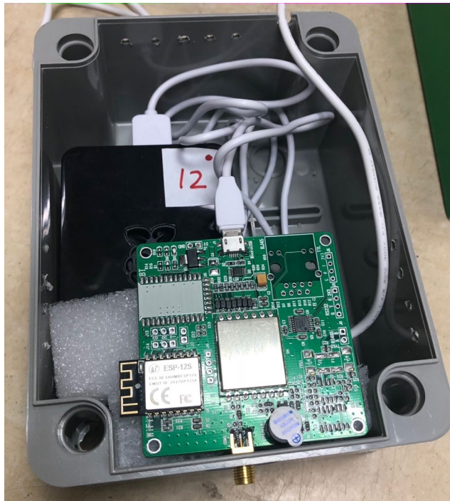
Figure 2.9.6: The Data Collection Terminal: integration of Raspberry Pi (IoT) and RFID reader module
