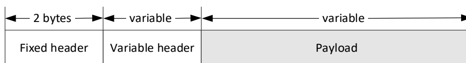
Figure 6.3.0-1: Format of MQTT Control Packet
