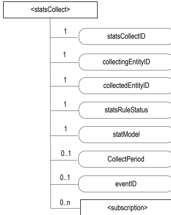
Figure 9.6.25-1: Structure of <statsCollect> resource
