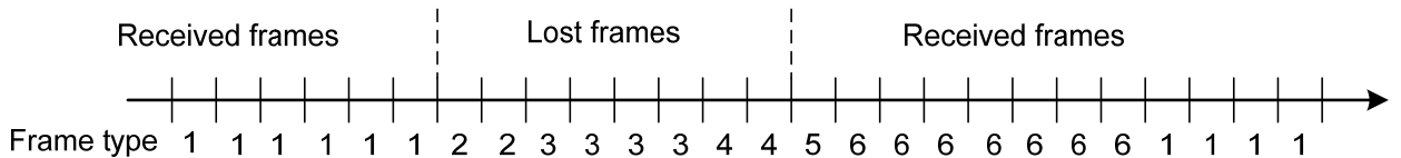
付図Ⅲ-1/J T-G 7 2 2 Time-line of frame types (ITU-T G.722)
